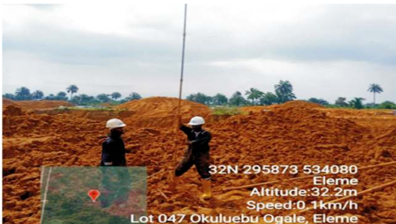
Plate 1.6: Collection of soil samples by manual slim hole augering during NOSDRA Close-out / Certification Sampling at Lot 047 -Okuluebu 2 (SPDC Ajeokpori Well Head 003), Ogale, Eleme L.G.A.
