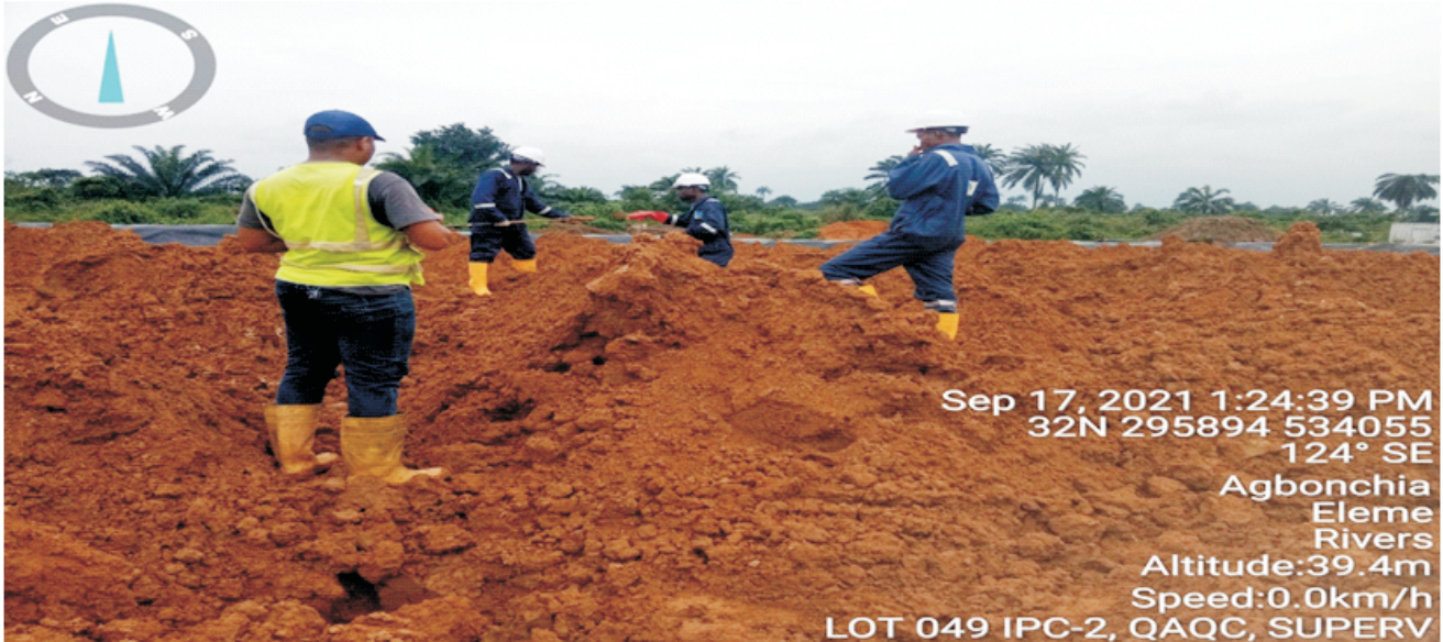
Plate 1.4: Quality Assurance / Quality Control (QA/QC) and Remediation Execution Officers from the Operations Unit of HYPREP collecting QAQC Monitoring Samples from treated soil volumes with the Contractor representatives at Lot 049 Okuluebu-Ogale, Eleme L.G.A). Remediation Contractor - ENVIRON CONSULT & REMEDIAL SERVICE LTD.
