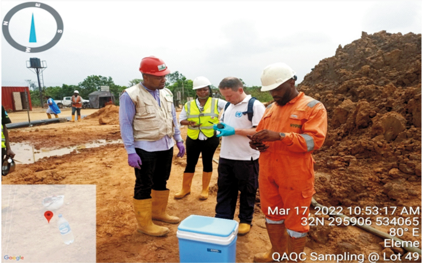
Plate 1.6: The UNEP Focal Person labelling a 60ml amber jar for collection of soil samples at Lot 049.(Lot 049 Contractor: ENVIRON CONSULT & REMEDIAL SERVICES LTD)
