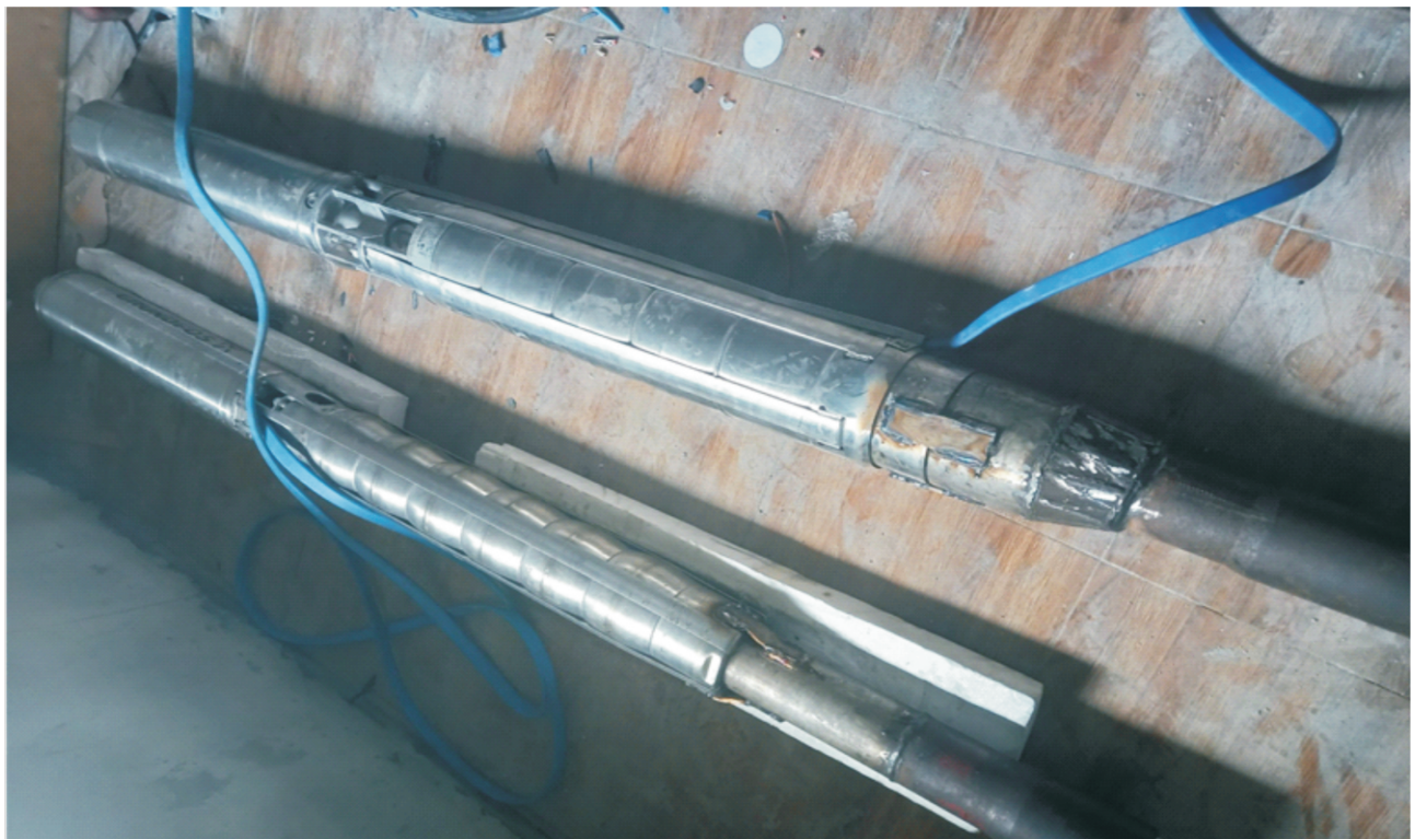
Submersible Pump 20Hp ready for installation at Barako Water Station
