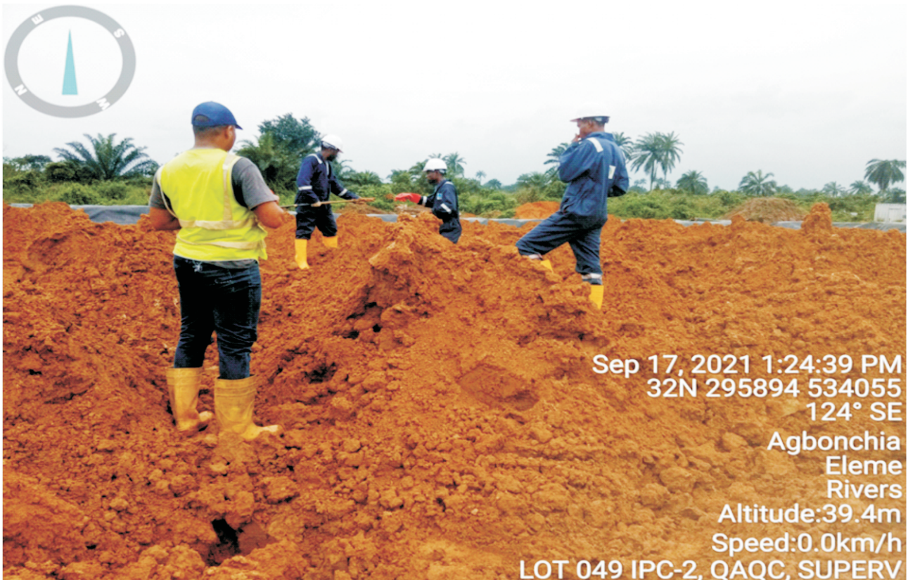
Plate 1.4: Quality Assurance / Quality Control (QA/QC) and Remediation Execution Officers from the Operations Unit of HYPREP collecting QAQC Monitoring Samples from treated soil volumes with the Contractor representatives at Lot 049 Okuluebu 2-Ogale, Eleme L.G.A). Remediation Contractor - ENVIRON CONSULT & REMEDIAL SERVICE LTD.
