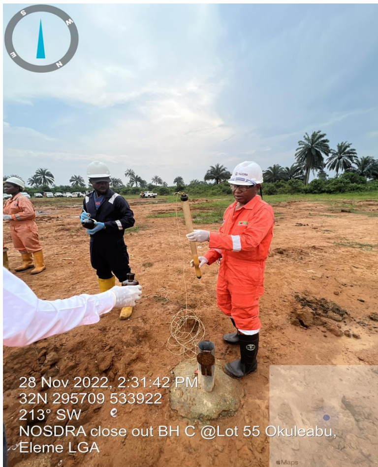
Plate 2.11: Groundwater Sampling from Monitoring Borehole done at Lot 055
