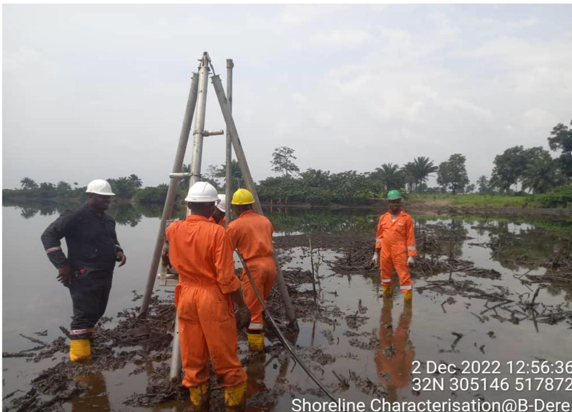
Plate 2.9: Setting up of Drilling Rig for Vibro-coring.
