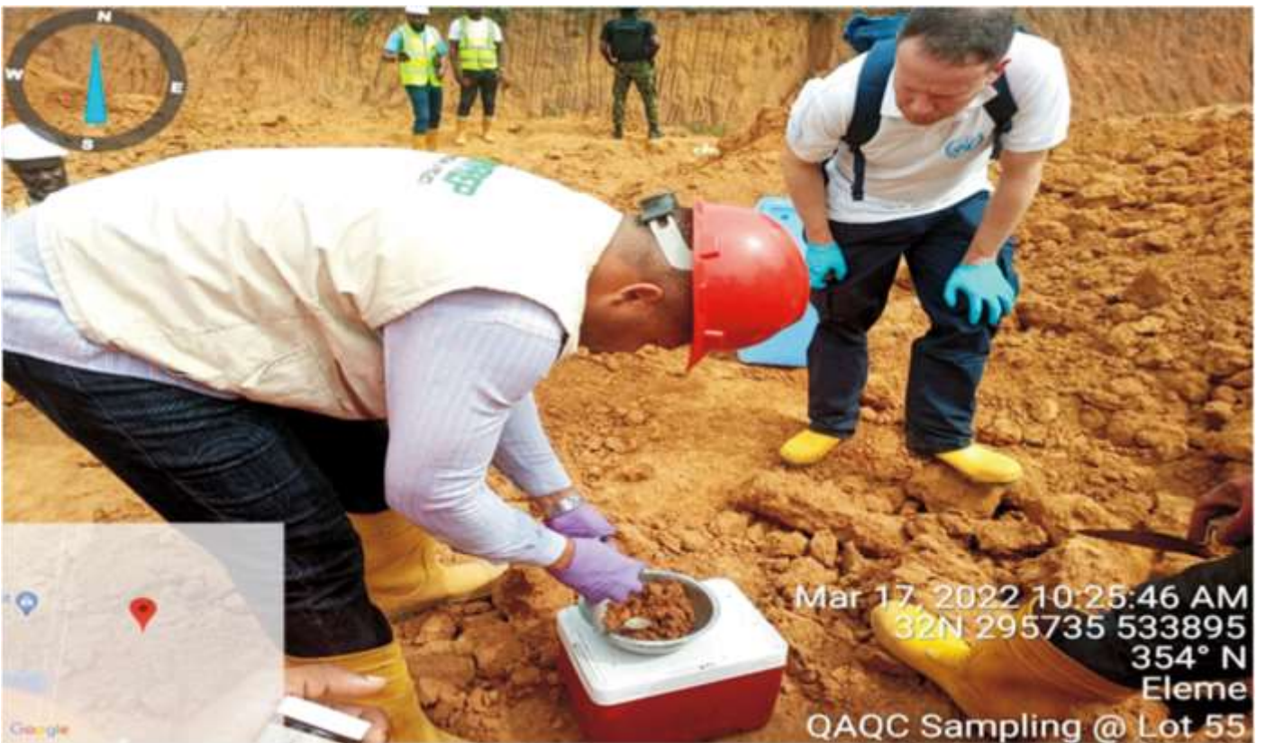
Plate 1.7: The Joint UNEP/HYPREP Team collecting soil samples from remediated stockpiles at Lot 055 in Okuluebu 2 (Ajeokpori Well 3), Ogale, Eleme L.G.A.(Lot 055 Contractor: ADG)
