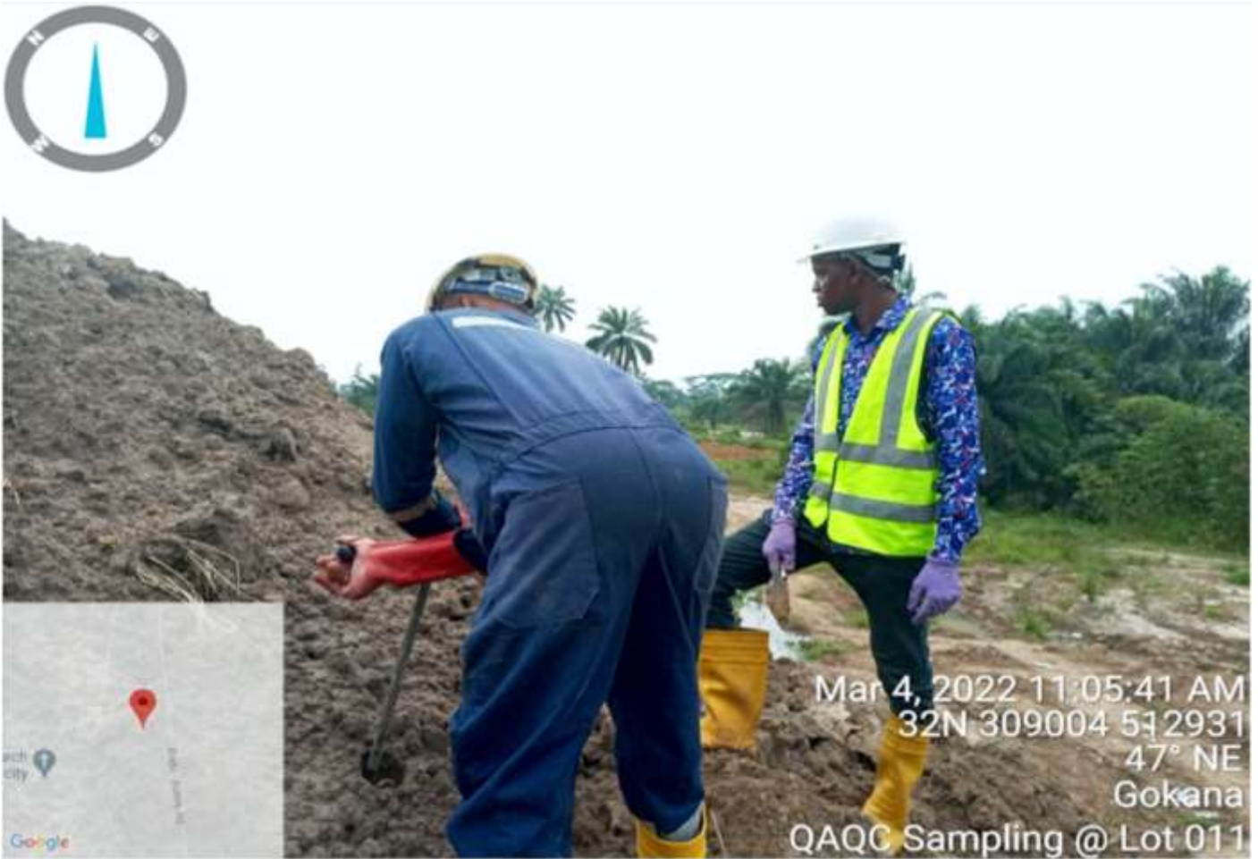
Plate 1.5: Scientific Officers from the Operations Unit of HYPREP collecting final QA/QC Monitoring Samples from treated soil heaps at Lot 011: Debon Section B, Bodo/ Mogho, Gokana L.G.A). Remediation Contractor -MOSVINNY NIGERIA LTD.
