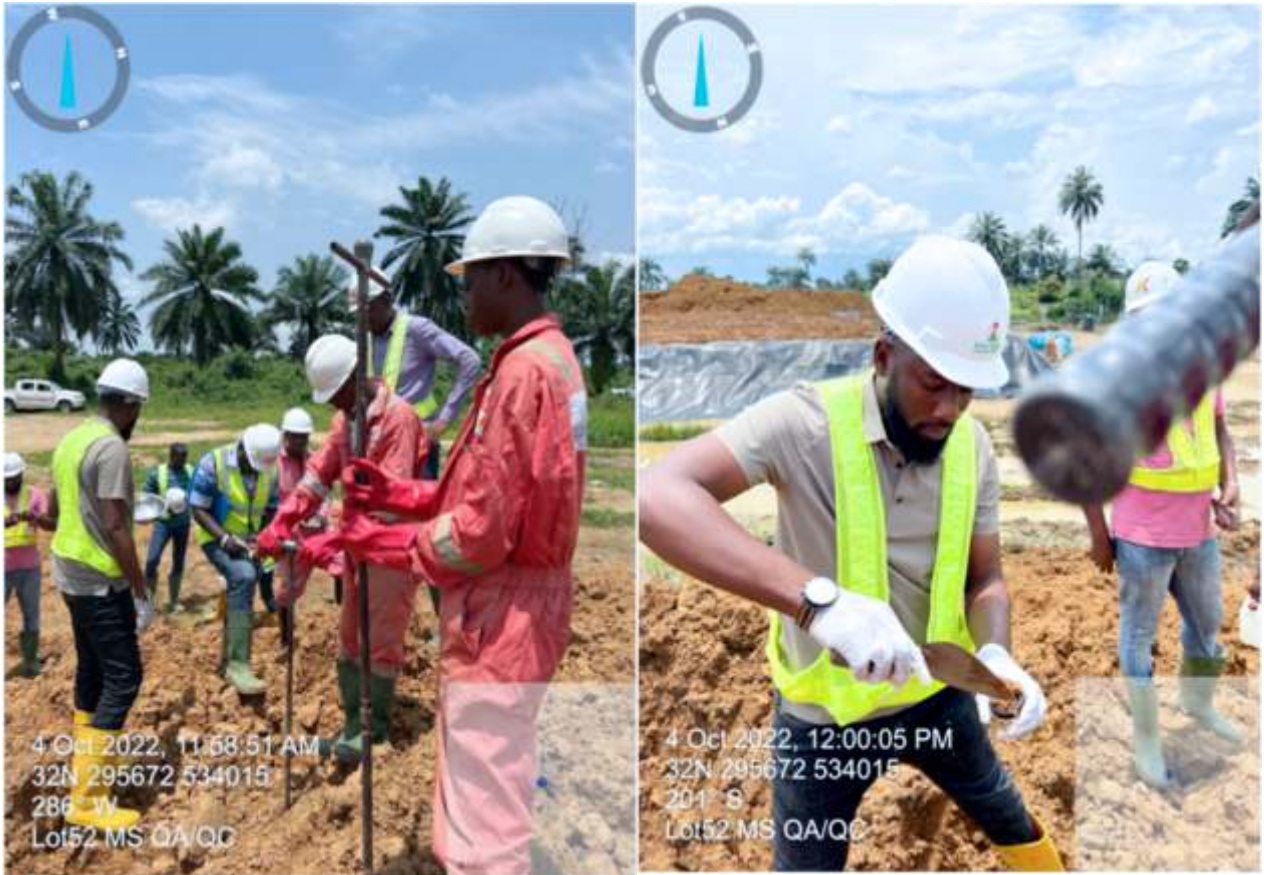
Plate 2.7: Scientific Officers of HYPREP QA/QC Team undertaking Sampling of Treated Soils at Lot 052 Okuluebu Ogale, Eleme LGA.
