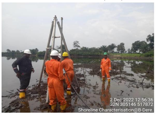
Plate 2.9: Setting up of Drilling Rig for Vibro-coring.
