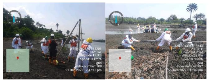
Plate 2.5: Core Retrieval Process in Operation Plate 2.6: Pulling out of the Cores from the barrels
