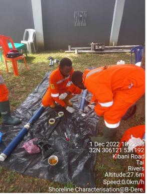
Plate 2.12: Cutting of Cores for sampling
