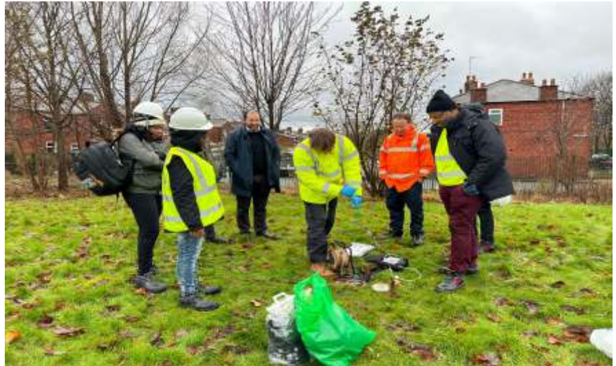
QA/QC Team Shown Borehole Measurement using Oil Water Interface Meter
