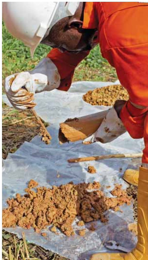
A soil sample is spread onto a polythene sheet
