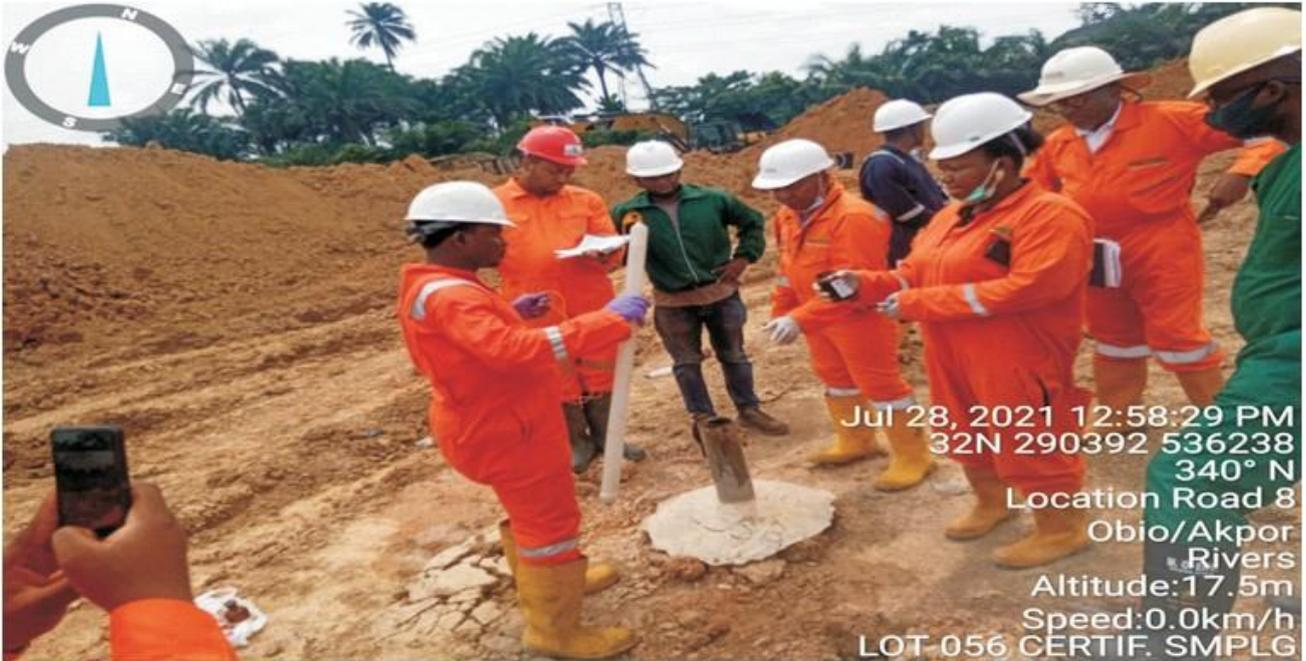
Plate 1.6: Collection of groundwater samples from remediation defensive / monitoring wells during the NOSDRA Close-out / Certification Sampling visit to Lot 056 at New Elelenwa Manifold area, Akpajo in Eleme L.G.A). Contractor: AWA ENGINEERING COMPANY LTD.
