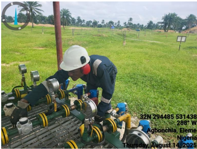
Plate5: Biosparging Setup at SMR Lot 015
